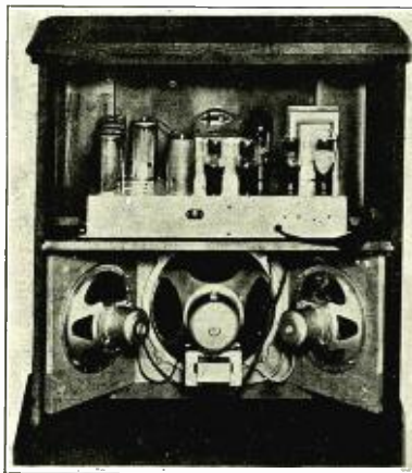
In this Sparton model, three speakers in an arc of a circle provide 155 square inches of sound-recording speaker surface. This application of principles in acoustical reproduction eliminates distortion and provides performance superior to dual-speaker arrangements.
